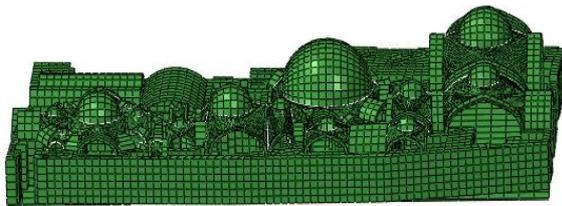
Fig. 8 Model made of bathroom in Abaqus environment
