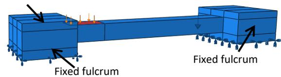
Fig. 5 Construction of boundary conditions and loading for reinforced concrete member
