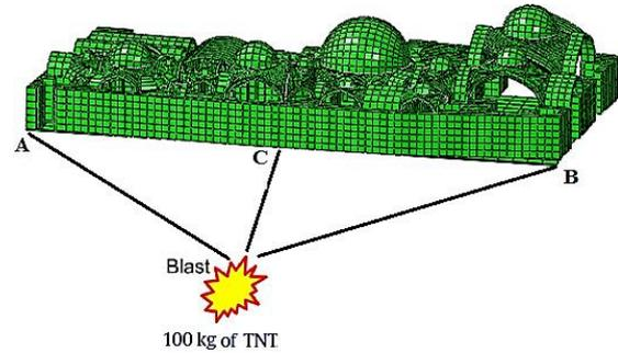
Fig. 12 Loading an explosion on Sheikh Baha'i's bath
