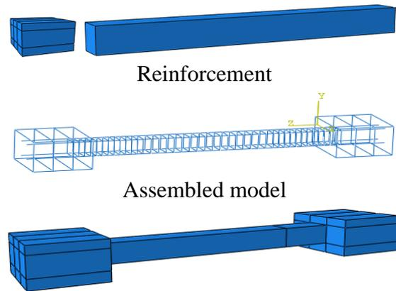
Fig. 4 Model assembly process
