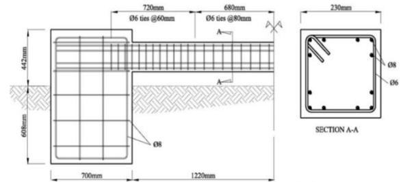
Fig. 1 General shape and specifications of laboratory sample [8]
