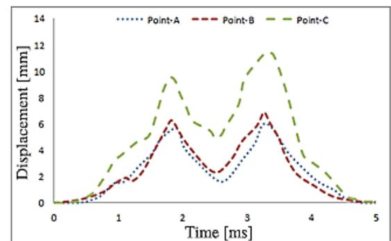
Fig. 13 Time history of the displacement under explosion
