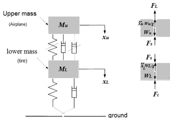
Fig. 4 Two-DOF model of the landing gear system and the free body diagram of the upper and lower mass.
