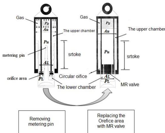
Fig. 2 The left image: Disable shock absorber, the right image: Semi-active shock absorber
