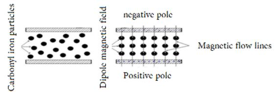
Fig. 1 The left image: particles in the absence of a magnetic field, the right image: particles in the presence of a magnetic field [9].
