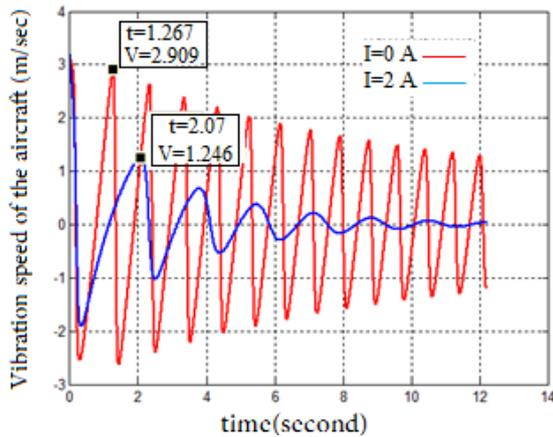
Fig. 6 The vibration velocity curve of the aircraft after the landing phase with a landing speed of  $v=3/2$
