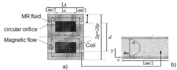
Fig. 3 (a) Schematic Valve MR, (b) velocity within circular orifice for Bingham plastic model
