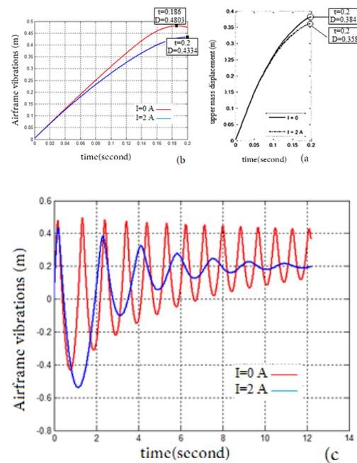
Fig. 5 Airplane vibration curve with landing speed of  $v= 3/2$ . a) The results of the fall test in the landing phase [11]; (b) results of landing phase; (c) results after the landing phase.
