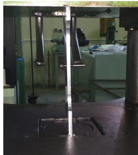
Fig. 3 Test specimen mounted on the fatigue test machine
