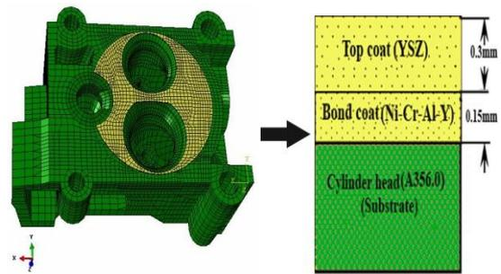
Fig. 2. The FE model of the coated cylinder head
