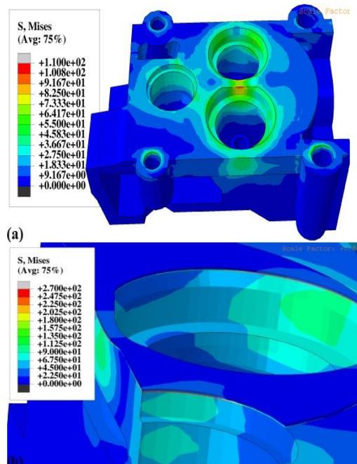
Fig. 8. The Von-Mises stress distribution in the coated cylinder head: (a) without TBC, (b) with TBC
