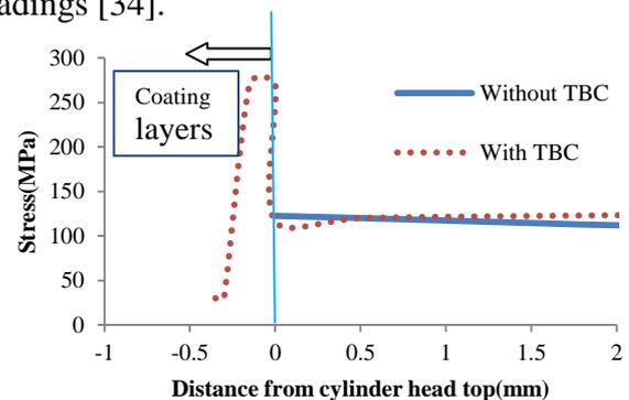
Fig. 9. The stress distributions through the thickness at the valve bridge
