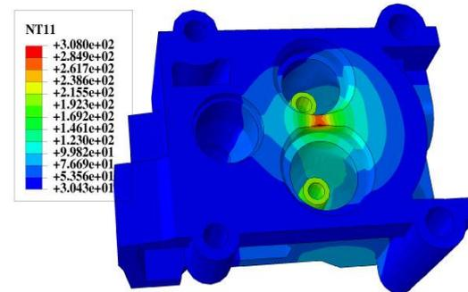
Fig. 3. The temperature distribution in the uncoated cylinder head [36]
