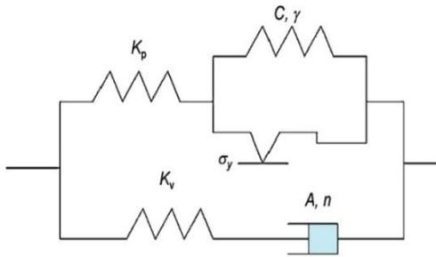
Fig.1. The two-layer viscoplasticity model [39]
