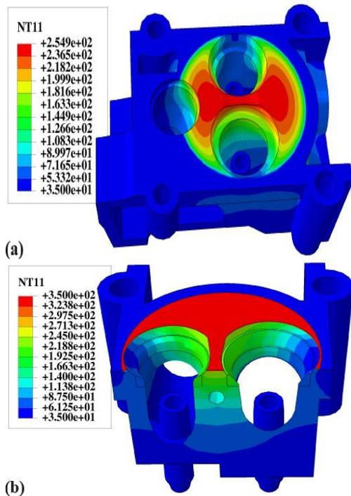
Fig. 4. The temperature distribution in the coated cylinder head: (a) without TBC, (b) with TBC
