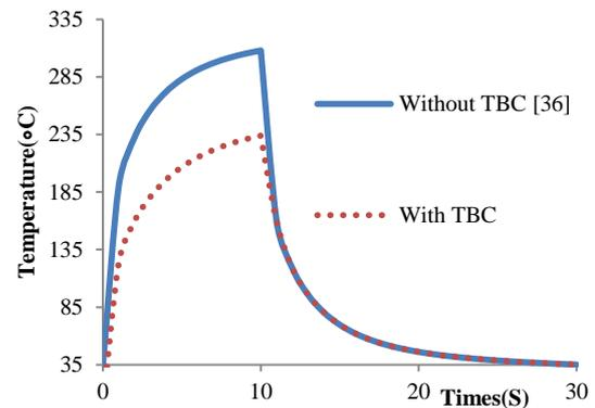
Fig. 5. The temperature at node 50420 versus time. The valve bridge is a crucial region [5]. Based on the source [1], the first fatigue cracks can be seen at the hottest spot of cylinder heads. This region is located in the valves bridge. The Temperature distribution through the thickness at the valve bridge are demonstrated in Figure 6.
