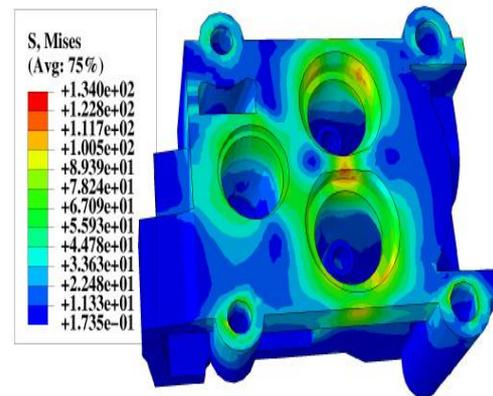
Fig. 7. The Von-Mises stress distribution in the uncoated cylinder head [36]
