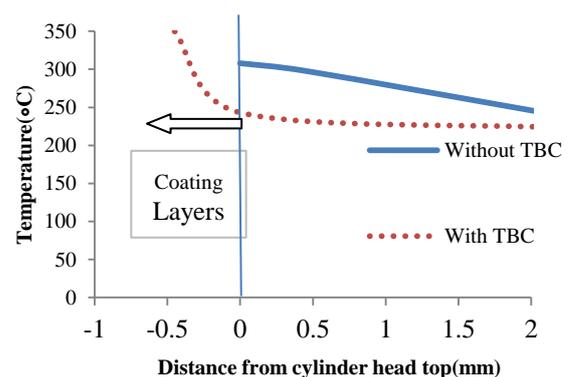
Fig. 6. The temperature distribution through the thickness at the valve bridge
