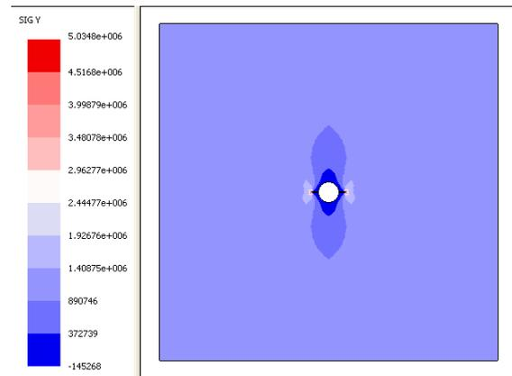
Fig. 6 Stress field around the hole and crack
