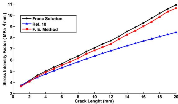
Fig. 7 Variations of SIFs at crack tip for various crack length with holes diameters 6 mm
