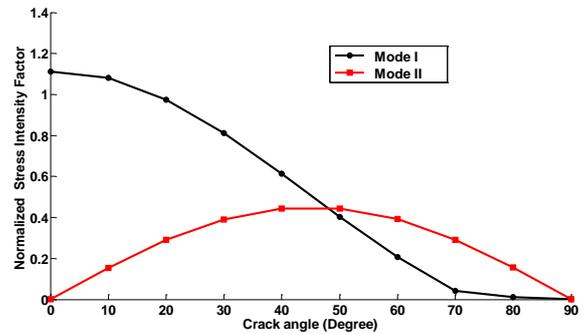
Fig. 12 Variations of the normalized SIFs in mode I and mode II for various crack angles
