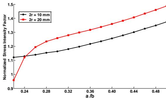
Fig. 10 Variations of the normalized SIFs for various  $a$  for hole diameters of 10 and 20mm
