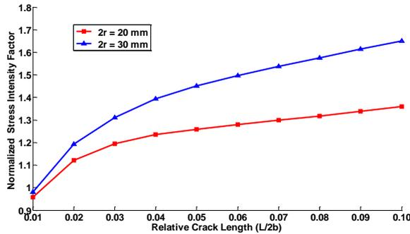
Fig. 9 Variations of the normalized SIFs at the crack tip for various crack lengths with hole diameters of 20 and 30 mm
