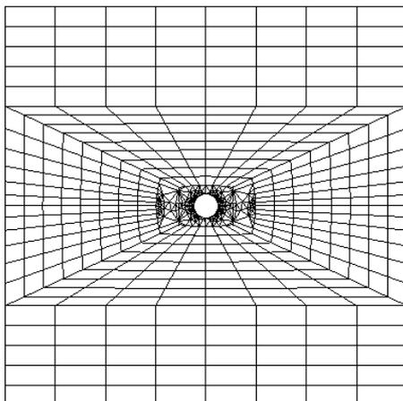
Fig. 4 The mesh plate before opening the crack
