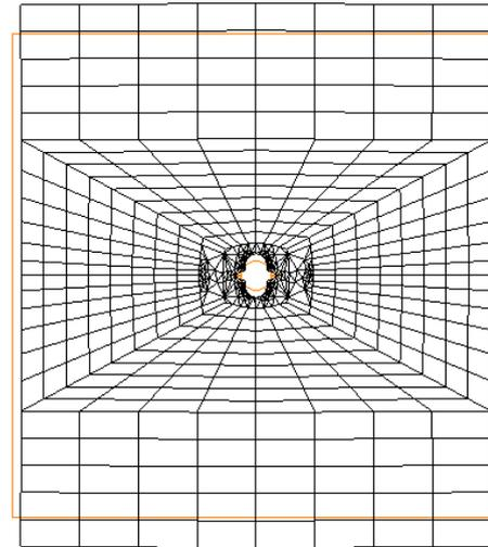
Fig. 5 The mesh plate after opening the crack
