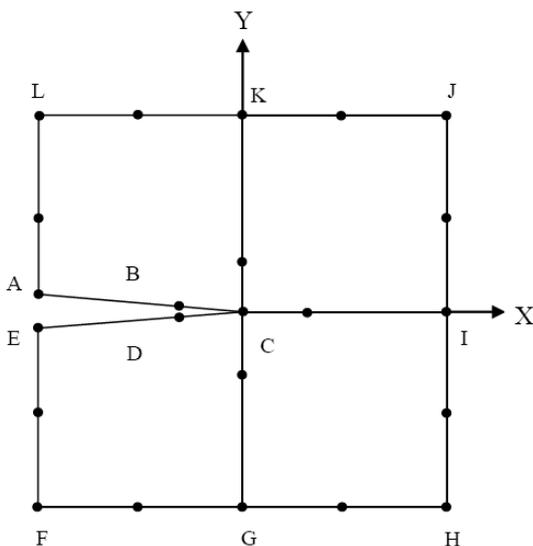
Fig. 2 Positions of mid-side nodes along the edges in singular elements around the crack tip
