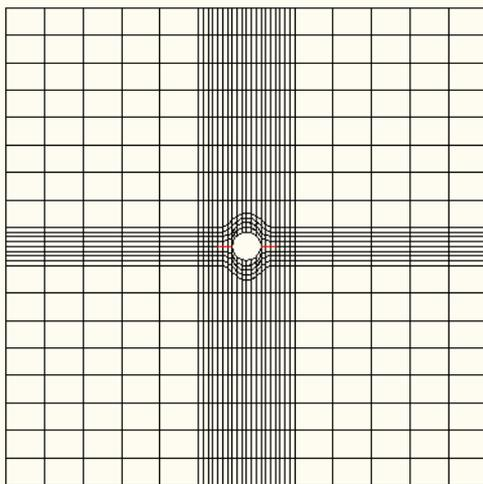
Fig. 3 Mesh with center hole plate in finite element method
