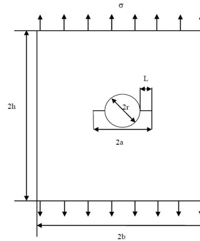
Fig. 1 The finite plate containing two symmetrical hole-edge cracks.
