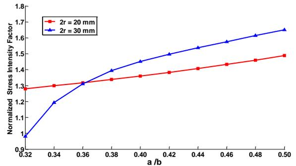
Fig. 11 Variations of the normalized SIFs for various  $a$  and different hole diameters of 20 and 30mm
