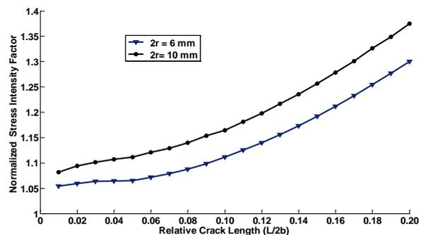
Fig. 8 Variations of the normalized SIFs at the crack tip for various crack lengths with hole diameters of 6 and 10 mm
